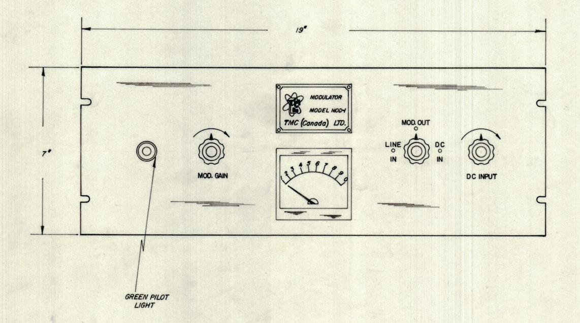
REQ. ITEM SYMBOL PART No. DESCRIPTION TMC (Canada) LIMITED ONTARIO STOCK SIZE AUDIO FREQUENCY MODULATOR FOR RFE EXCITER Moder DRAWN HEAT TREAT. SPEC. A-10 196
