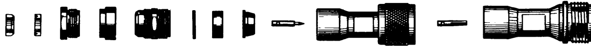
*GLAND *GASKET NUT #1 CAP NUT #2 WASHER GASKET CLAMP MALE CONTACT PLUG BODY FEMALE CONTACT JACK BODY (CROSS SECTION VIEWS)
