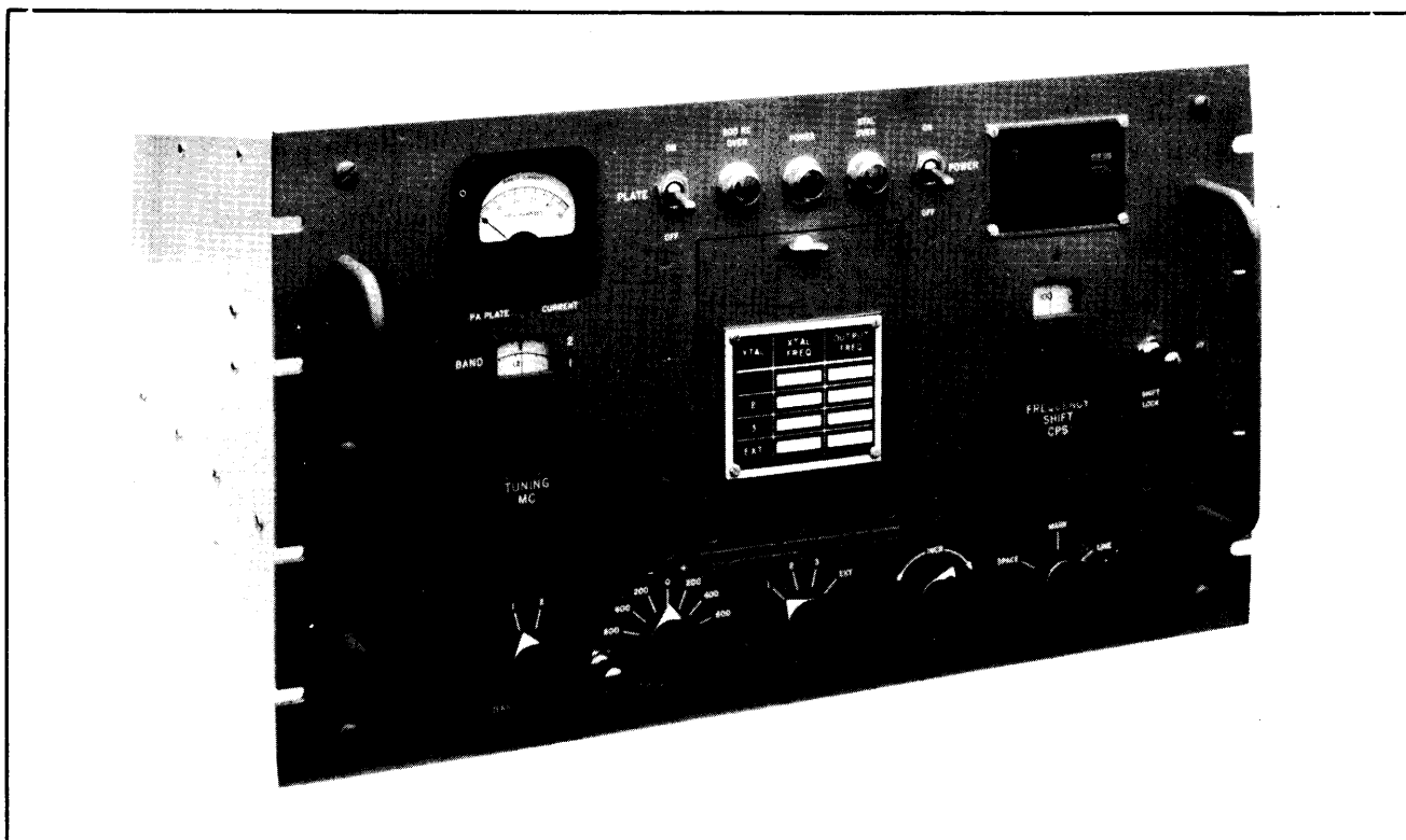
Figure 1-1 Frequency Shift Excitor Model XFK - Front View Showing Controls and Crystal Oven Access Door
