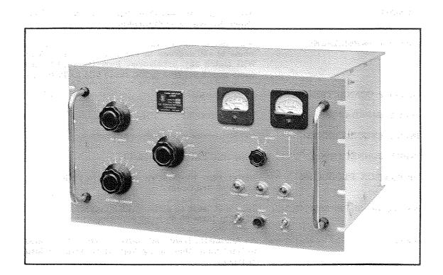
The TMC Model PAL-350, Linear Power Amplifier is a conservatively rated general purpose amplifier providing 300 watts PEP output over the frequency range 2 to 32 Mcs.
