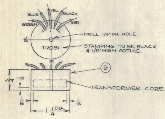
NOTE: ALL LEADS 1-1/2"LONG OVERALL AFTER POTTING WIRE PROJECTS 1/4" FROM SLEEVE \$ 15 TINNED.
