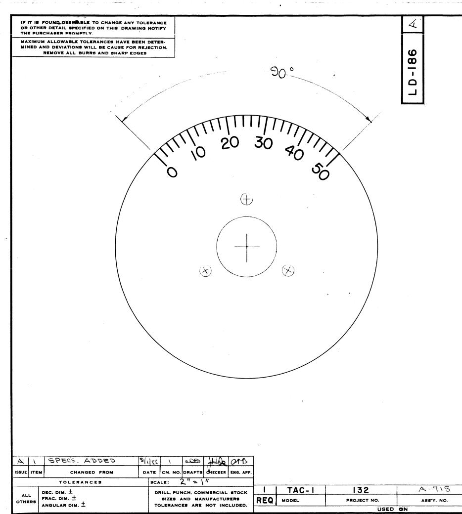
RANGE OF INSCRIPTION - O TO 50 CW LINEAR TOTAL QUAN, OF SCALE DIVISIONS - 25 DIAMETER - 2 3/4" OVERALL CENTER HOLE - 5/8" DIA. 3 MTG HOLES - 1/8" DIA. ON 1/2" RADIUS
