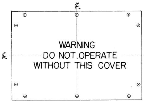
ALL LETTERING TO BE 1/4" HIGH RED GOTHIC MARKING PROCESS: AS PER TMC SPECIFICATION S-727
