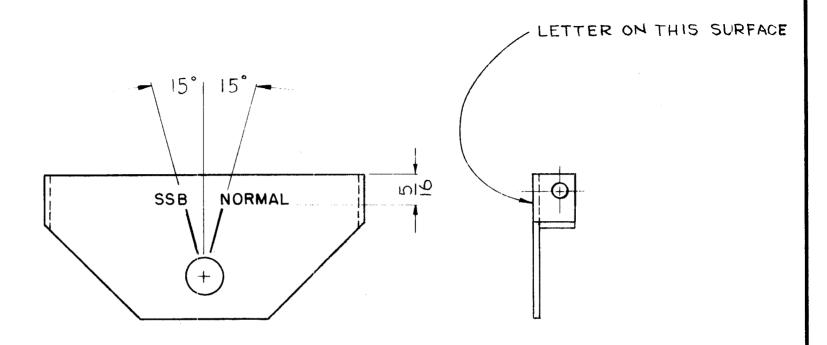
MARKING PROCESS: AS PER TMC SPECIFICATION S-727.
