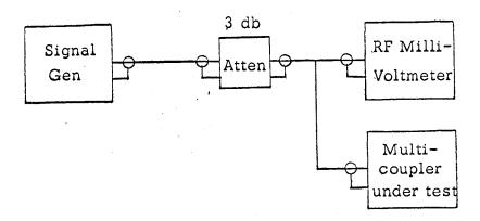
Note: Make leads from Attenuator to Multicoupler and RF Millivoltmeter probe as short as possible.
