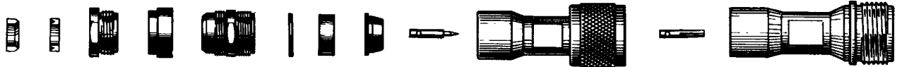
*GLAND *GASKET NUT #1 CAP NUT #2 WASHER GASKET CLAMP MALE CONTACT PLUG BODY FEMALE CONTACT JACK BODY
