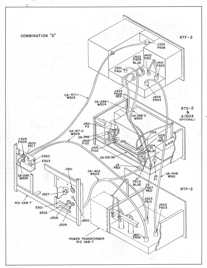
Figure D-2-3 Cabling Connections Model GPT-750D2
