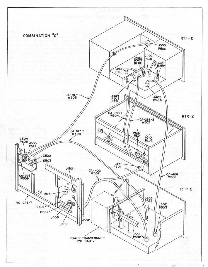
Figure C-3-1 Cabling Diagram Model GPT-750C2
