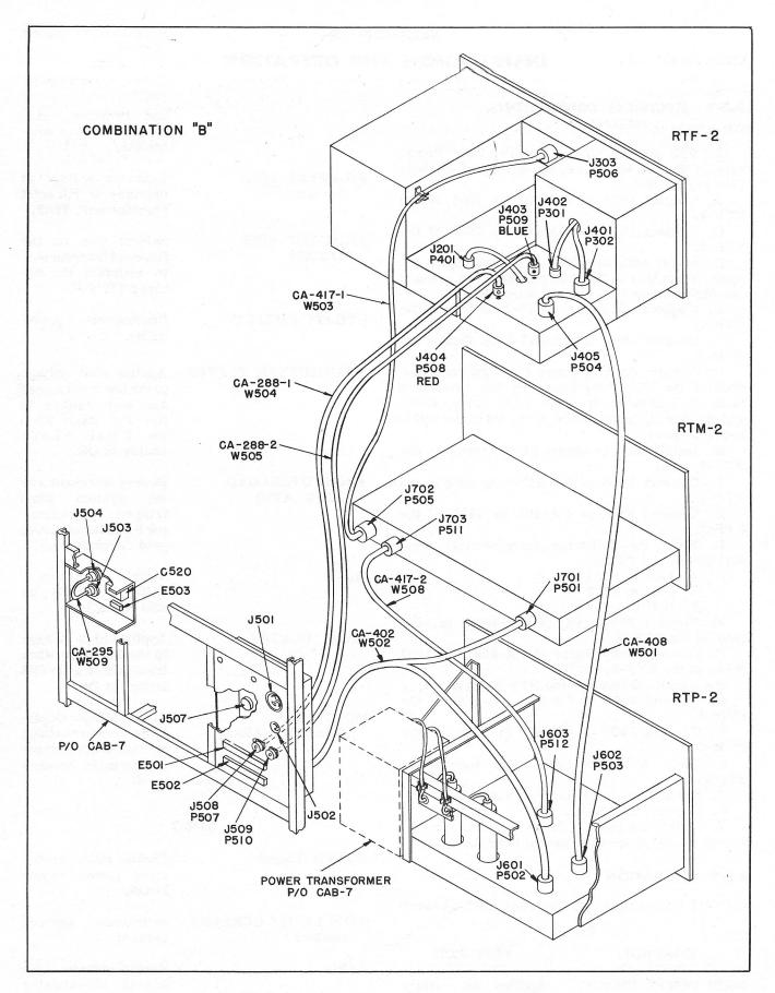
Figure B-3-1 Cabling Diagram Model GPT-750B2
