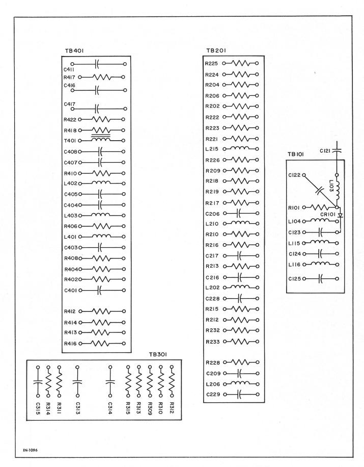
Figure E-8 Terminal Board Layout Model RTF-2
