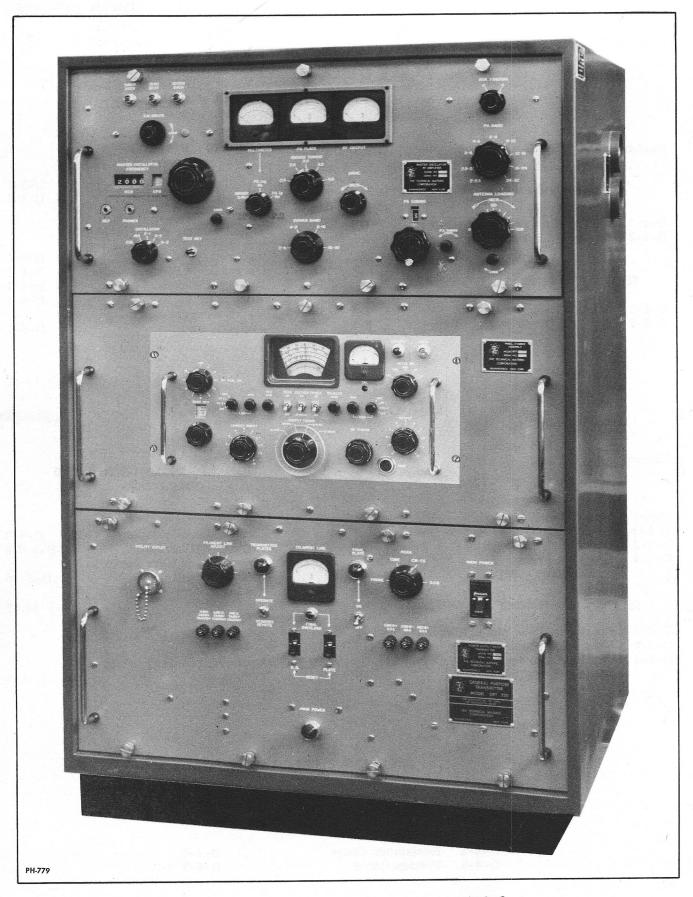
Figure D-1-1 Front View Model GPT-750D2
