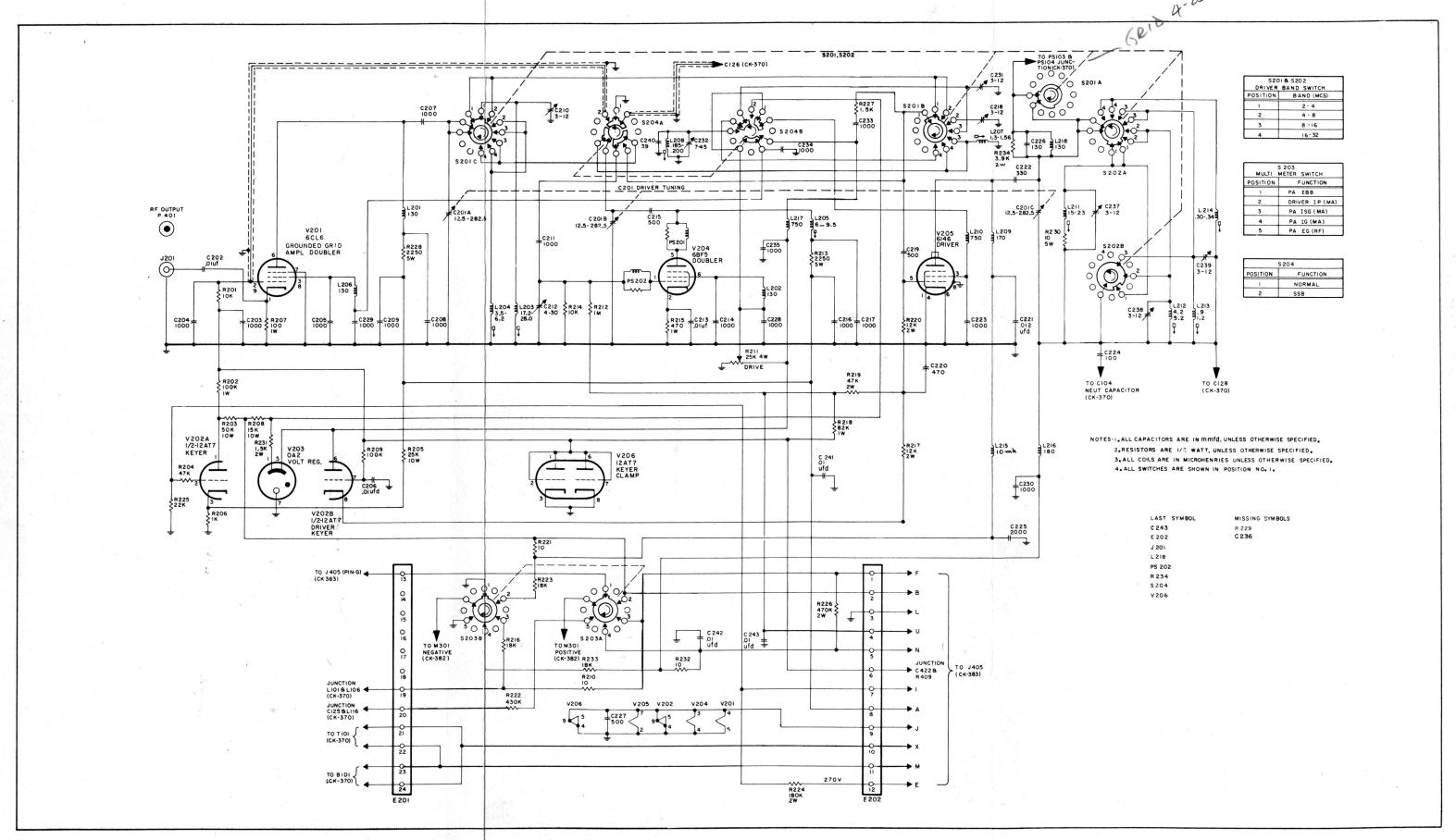
Figure E44 Schematic Diagram, Multiplier Section, Model RTF-2
