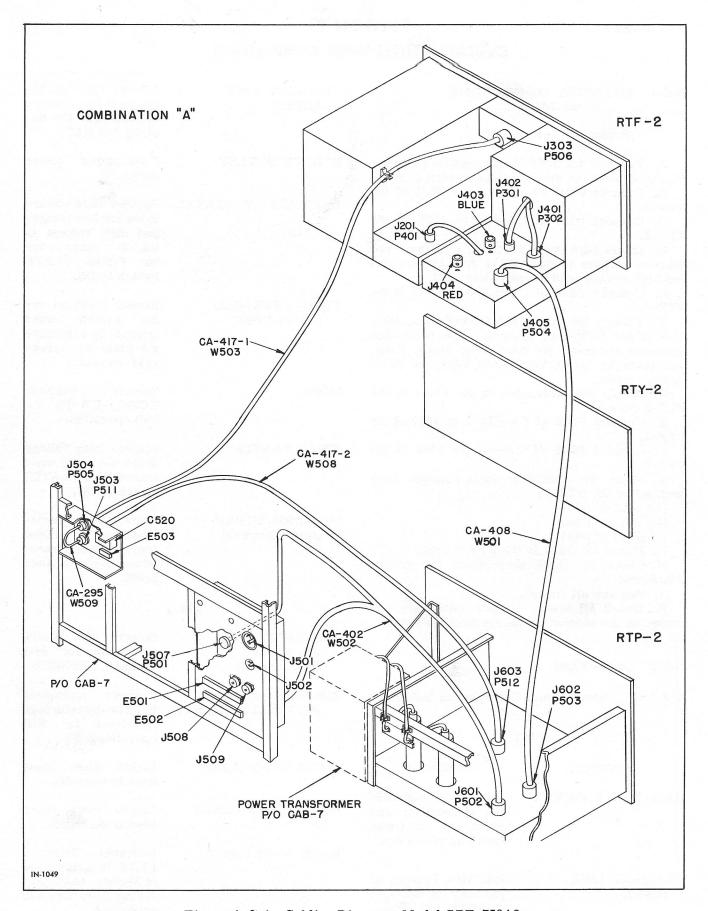
Figure A-3-1 Cabling Diagram Model GPT-750A2
