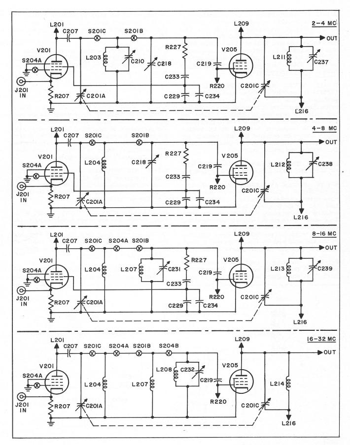
Figure G-2-8 Simplified Schematic Diagram Multiplier with Switch S204 in SSB Position
