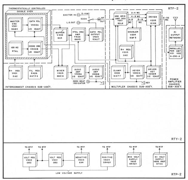
Figure A-1-2 Block Diagram Model GPT-750A2
