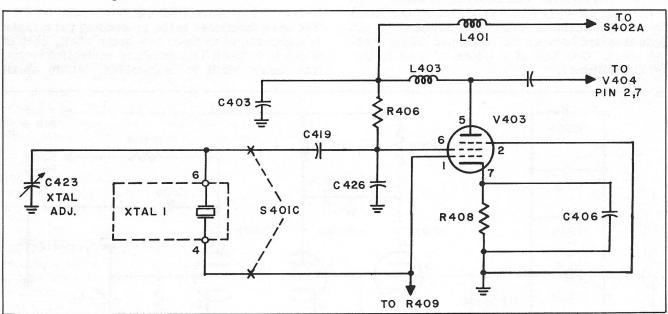
Figure G-2-3 Simplified Schematic Diagram Crystal Oscillator/Amplifier
