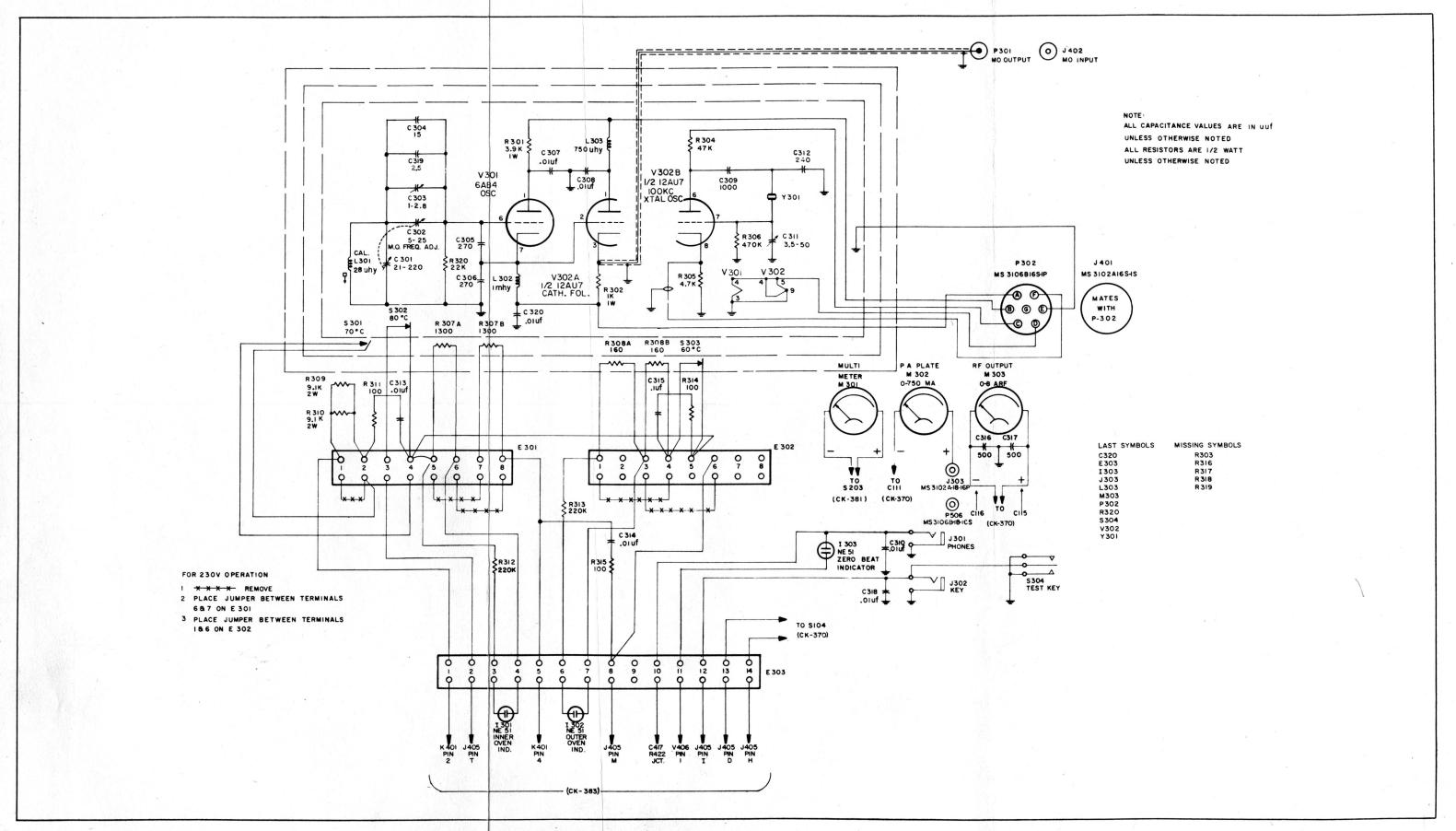
Figure E45 Schematic Diagram, Master Oscillator and Front Panel, Model RTF-2
