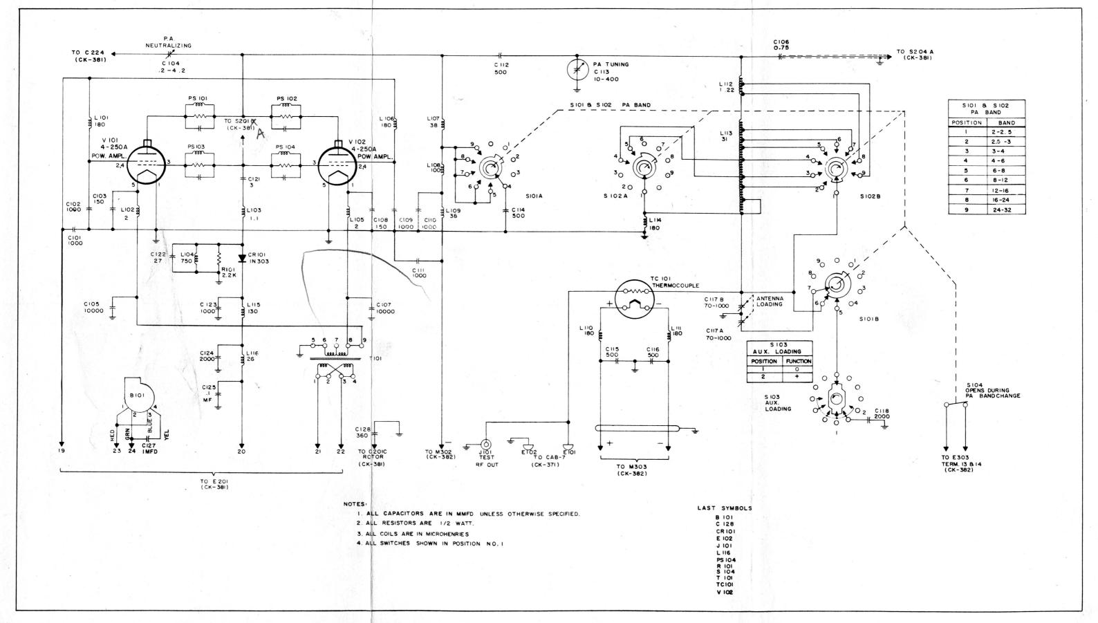
Figure E43 Schematic Diagram, Power Amplifier Section, Model RTF-2
