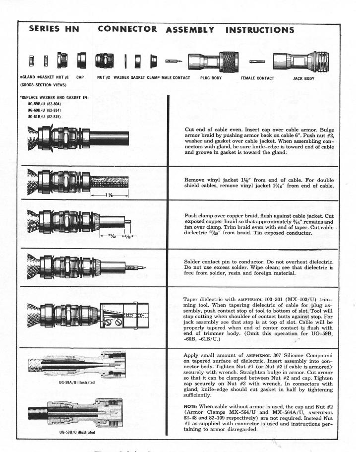
Figure G-3-4 Connector Assembly Instructions
