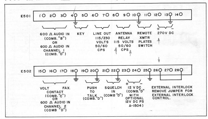
Figure G-3-3 Terminal Board Connections CAB-7
