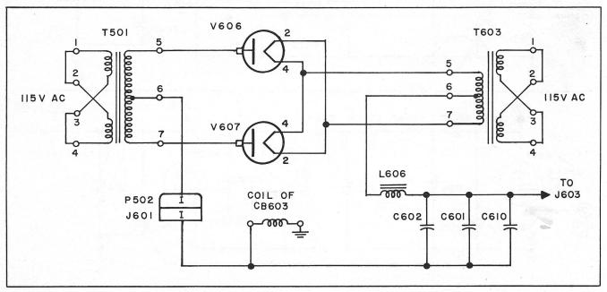
Figure G-2-9 Simplified Schematic Diagram High Voltage Supply
