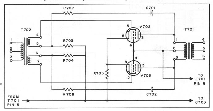
Figure B-2-2 Simplified Schematic Diagram Modulator Driver
