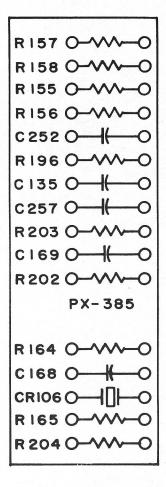
Figure E-36 Terminal Board Layout Exciter Unit
