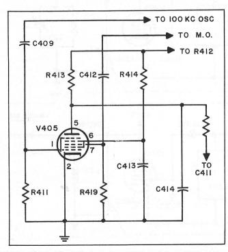
Figure G-2-5 Simplified Schematic Diagram Mixer Circuit
