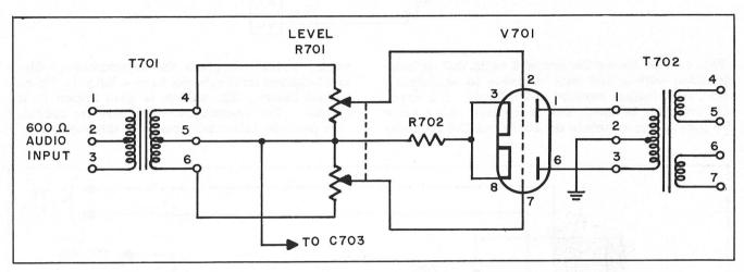
Figure B-2-1 Simplified Schematic Diagram Audio Amplifier
