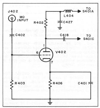
Figure G-2-2 Simplified Schematic Diagram Buffer Stage
