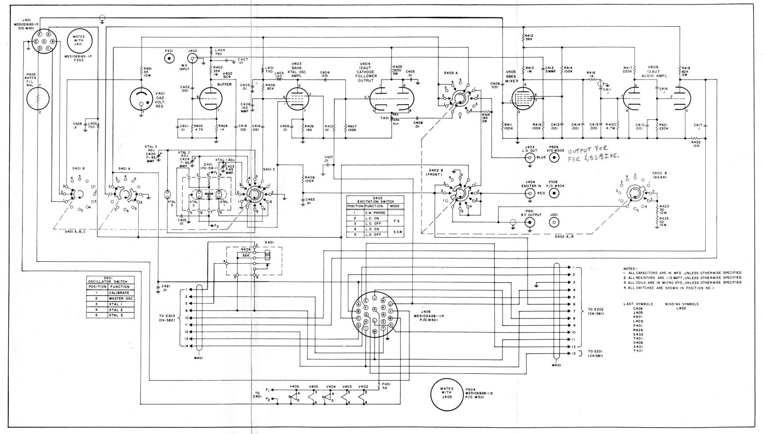
Figure E46 Schematic Diagram, Interconnect Chassis, Model RTF-2
