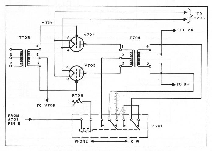
Figure B-2-3 Simplified Schematic Diagram Modulators
