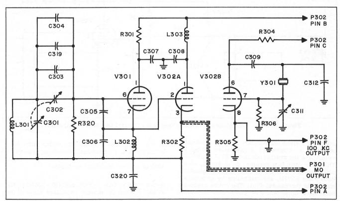
Figure G-2-1 Simplified Schematic Diagram Oscillator Circuits
