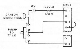
This circuit shows the use of 6 volts D.C. in conjunction with a 220 ohm resistor to maintain a D.C. microphone current of 20-30 ma. If a lower D.C. voltage is used, the resistance value must be lowered to maintain the 20-30 ma D.C. current
