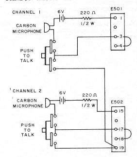
This circuit shows the use of 6 volts D.C. in conjunction with a 220 ohm resistor to maintain a D.C. microphone current of 20-30 ma. If a lower D.C. voltage is used, the resistance value must be lowered to maintain the 20-30 ma D.C. current rating which energizes the microphone. Since most carbon microphones have a built-in "pushto-talk switch, this switch is also shown in the circuit. The transmitter may now be operated on a push-to-talk basis from the microphone.
