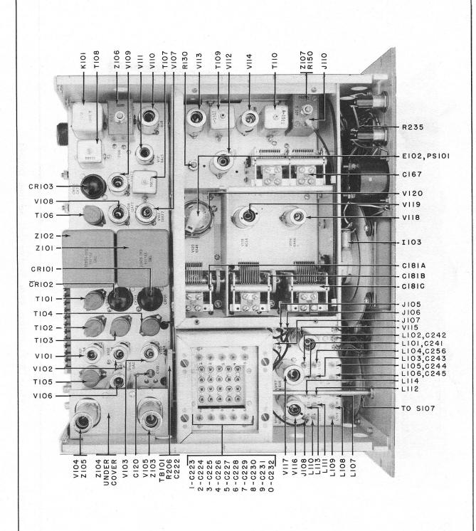
Figure E-31 Bottom View Exciter Unit Sections Defined
