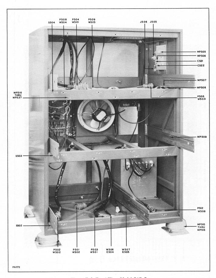
Figure E-1 Front View Model CAB-7
