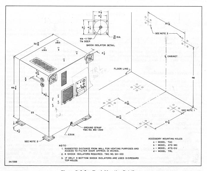
Figure G-3-2 Shock Mounting Details
