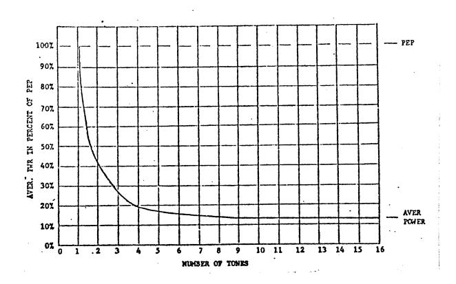
Figure 3-1. Ratio of Average Power and PEP As a Function of Tones
