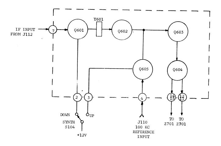
Figure 4-2. Carrier Filter, 7601, Simplified Block Diagram
