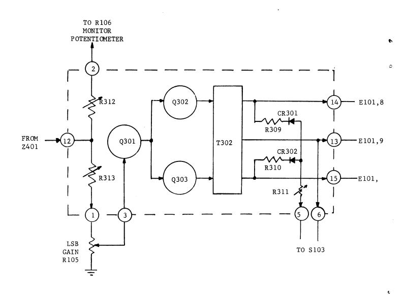
Figure 4-6. LSB Line Amplifier, Z301, Simplified Block Diagram
