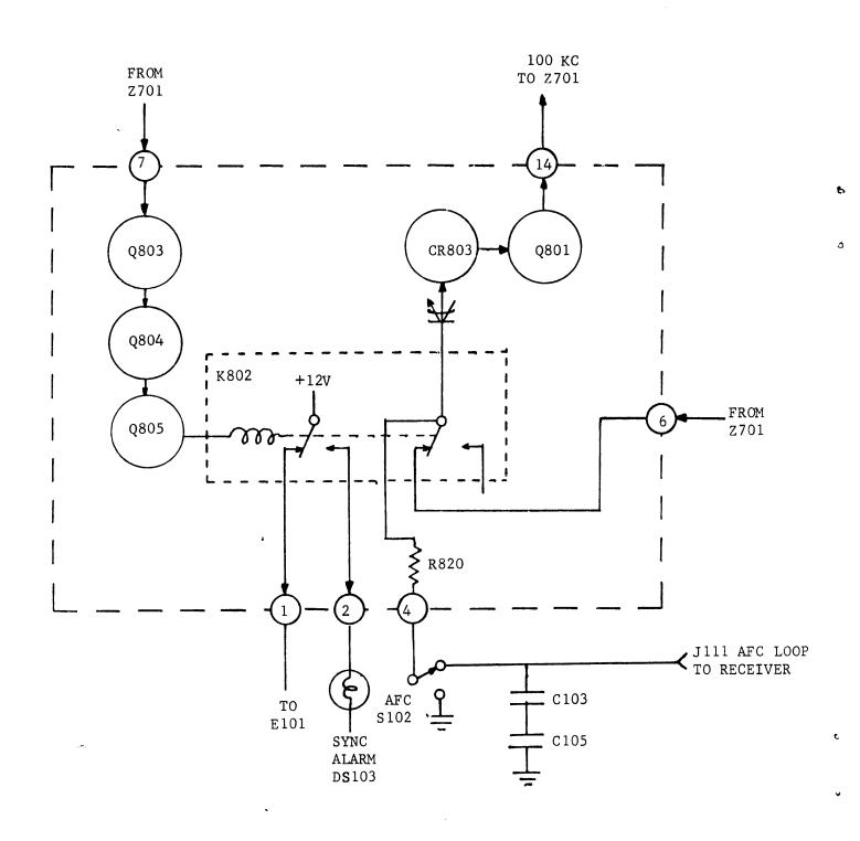
Figure 4-5. Crystal Oscillator, 7801, Simplified Block Diagram
