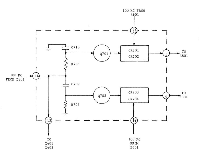
Figure 4-4. Phase Detector, Z701, Simplified Block Diagram
