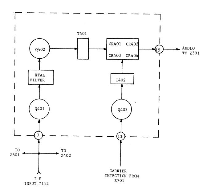
Figure 4-1. LSB Product Detector, Z401 Simplified Block Diagram.
