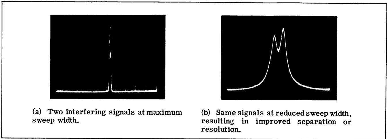
Figure III-7. Resolution of Interfering Signals.
