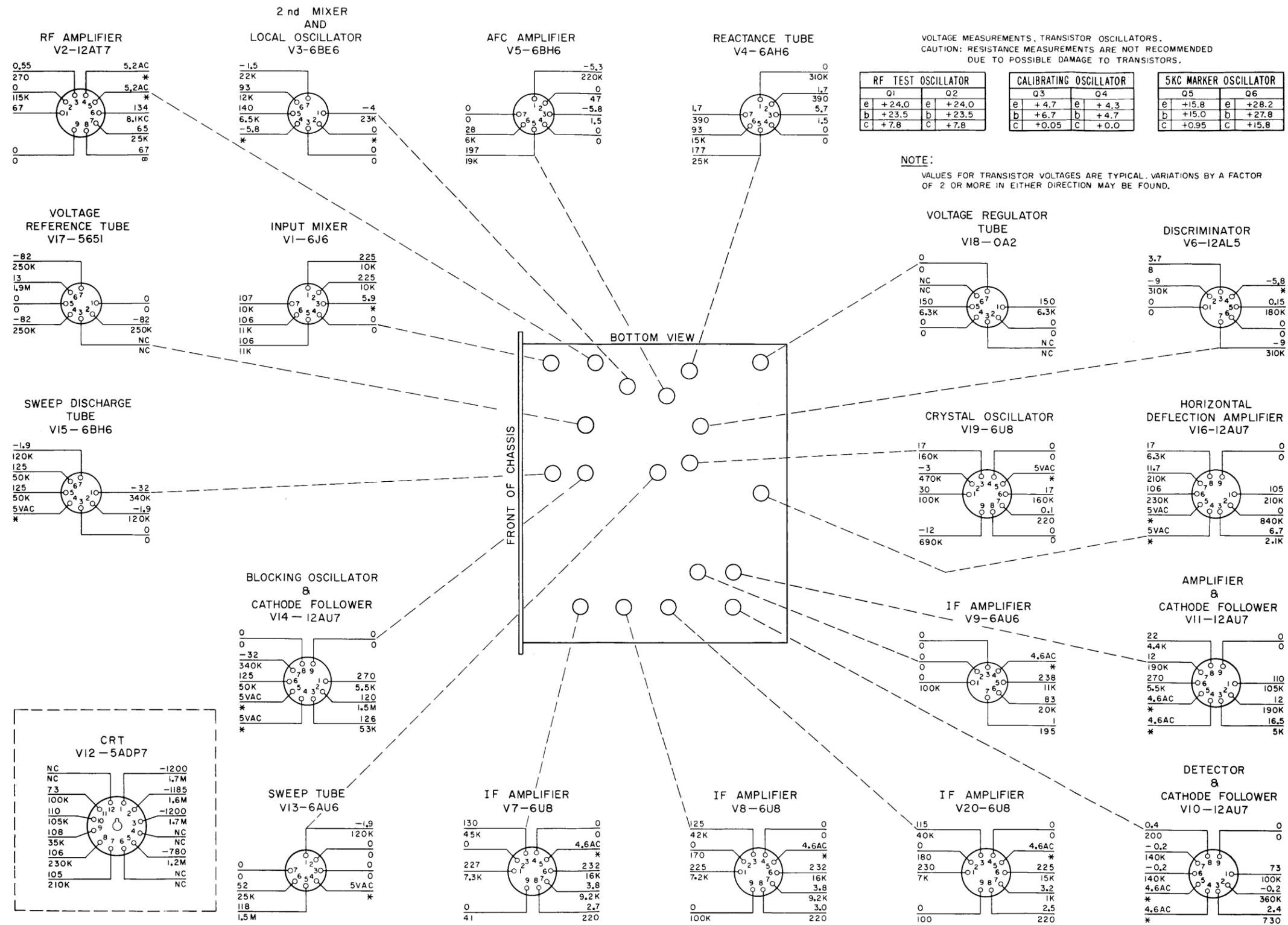
Figure V-2. Voltage and Resistance Chart, Model SB-12a
