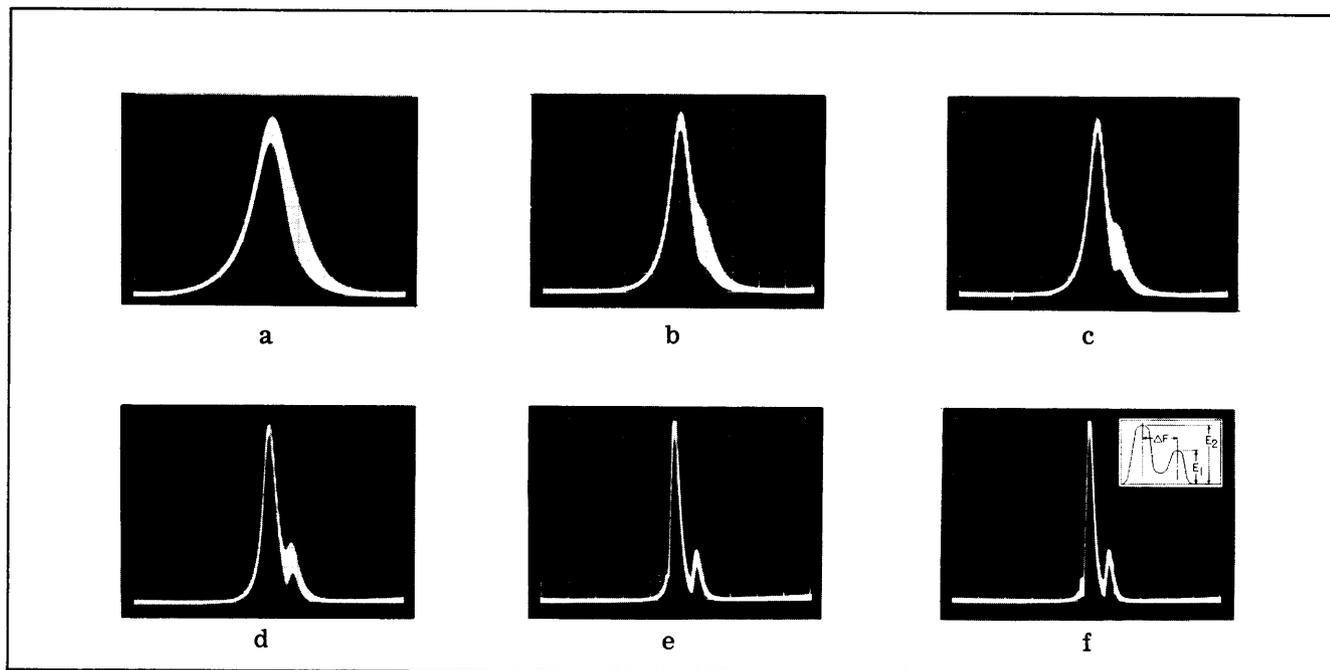
Figure III-3. Resolution of Signals of Unequal Amplitude.
