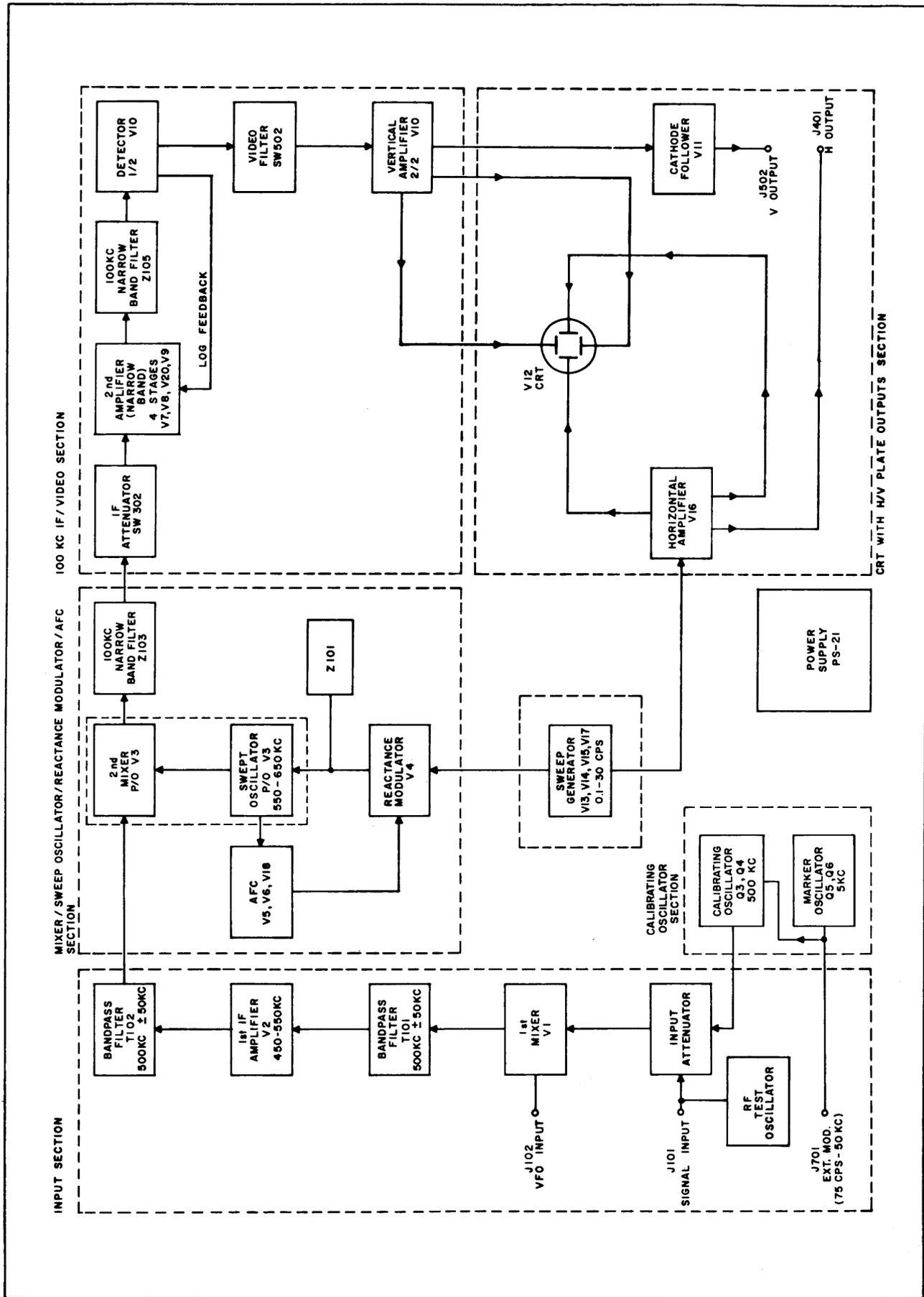
Figure IV-1. Block Diagram, Model SB-12aS.
