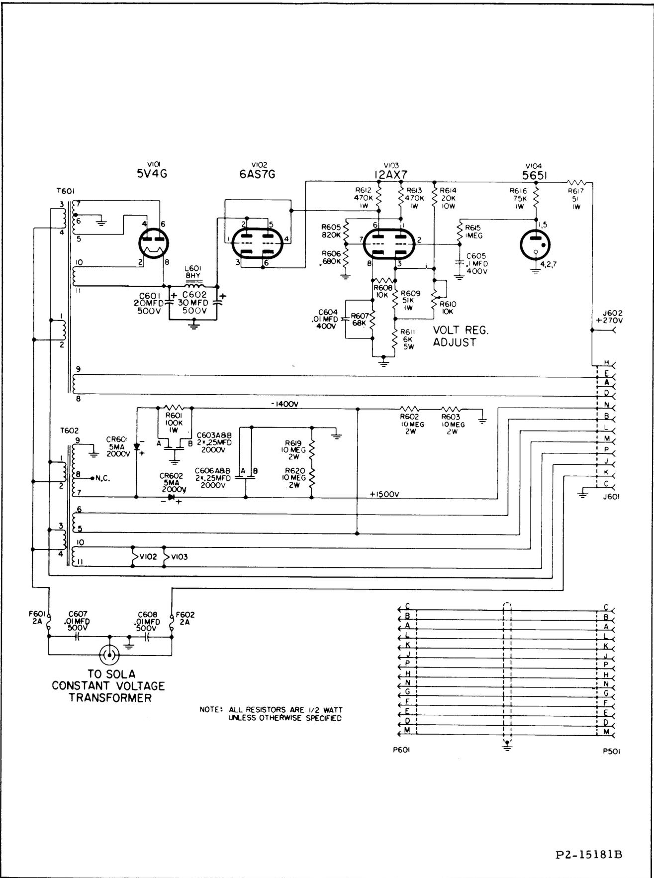
Schematic Diagram, Power Supply, Model PS-12
