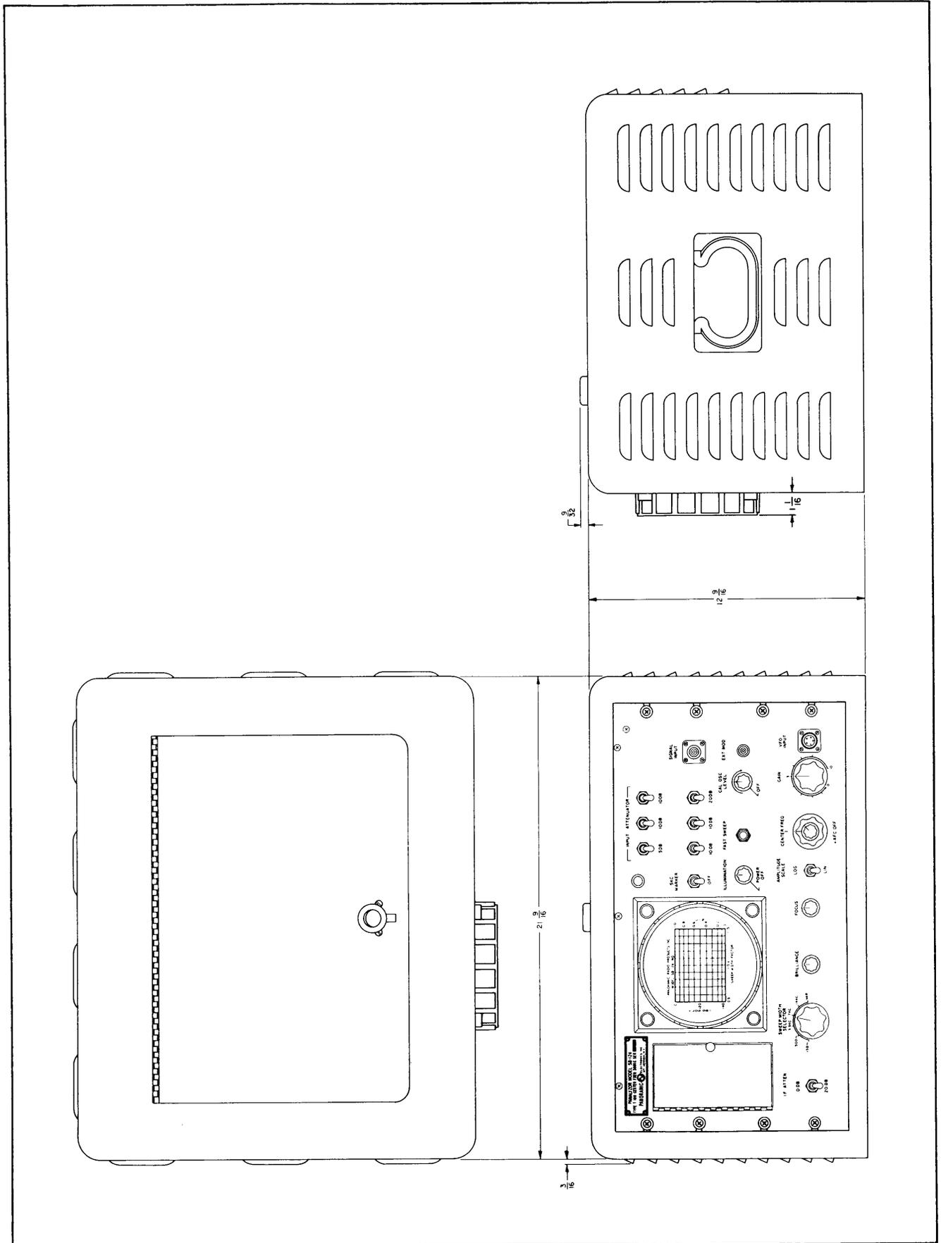
Figure II-4. Outline Dimensional Drawing, Model SB-12a in Cabinet.
