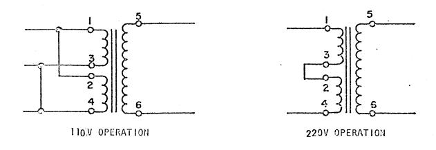
Figure 2-1. 110% to 220V TRANSFORMER WIRING DIAGRAM
