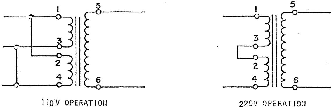
Figure 2-1. 110V to 220V TRANSFORMER WIRING DIAGRAM
