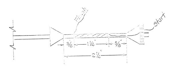
Forms should be waxed to prevent wire slippage and a slow winding speed should be used.
