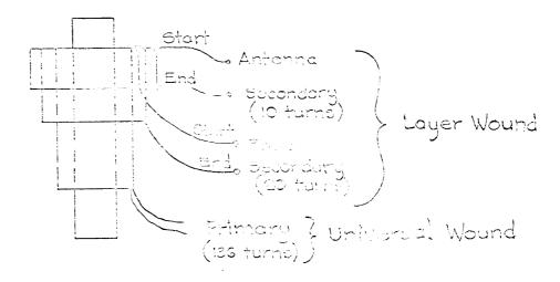
LB5 and LC5 coils are wound like LA5 with the exception that no antenna winding is needed.
