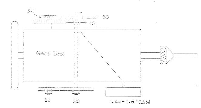
2. Coil forms used was XXX Natural Paper Base Bakelite with an O.D. of 1/4 inches and an I.D. of 3/16 inches. Coil forms were cut to 2 1/4 inches long. Coils were wound on form between two imaginary lines, one 3/8 inch from top of form with the other 5/8 inch from bottom of form. A sketch of form mounted in winder is shown below.
