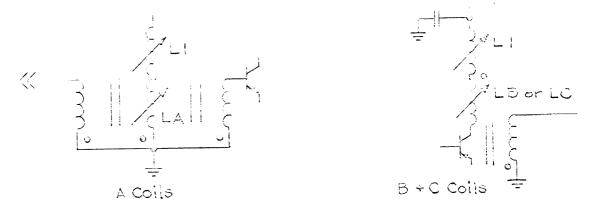
The sketch uses the dot convention where the dot is shown on the coil at the beginning of coil winding.
