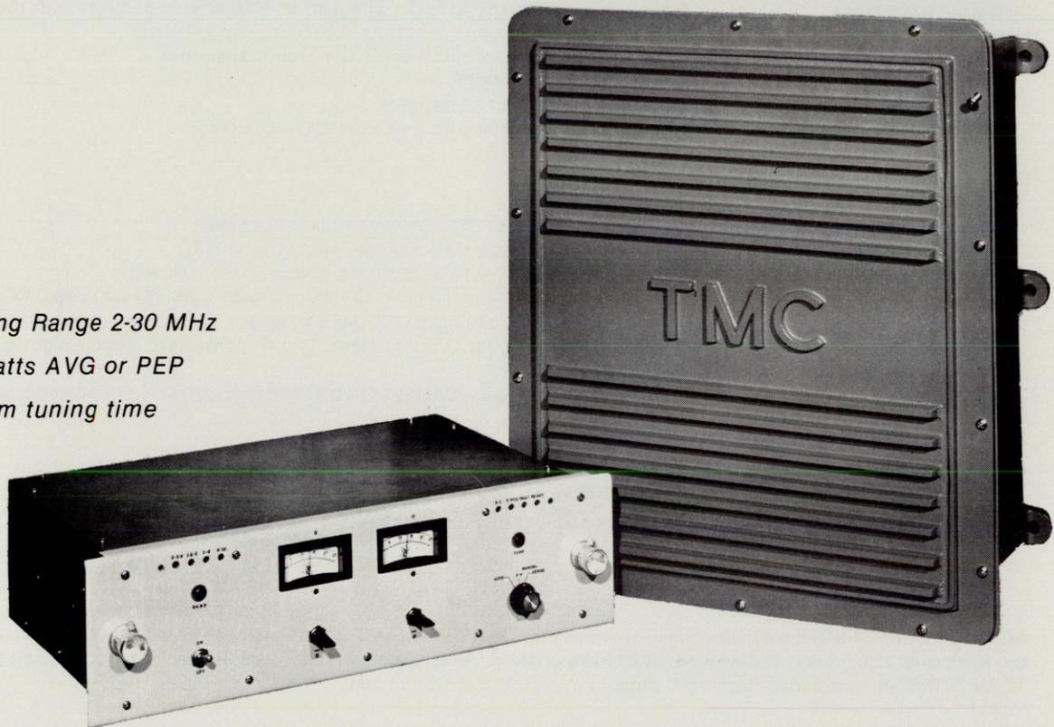
The ATS-3 antenna tuning system is a highly versatile automatic device which will remotely tune a 35 foot shipboard antenna to match the 50 ohm output of a 1 KW transmitter over the range of 2-30 Mhz. It will also tune into a long wire antenna as short as fifteen feet depending on frequency and antenna configuration.
