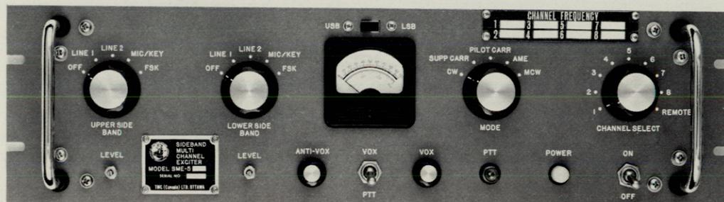
The SME-5 is a fully transistorized, eight channel ISB exciter with a frequency range of 2 to 30 MHz. It provides up to 100 milliwatts PEP output as drive power for an associated linear amplifier. Capable of operating in all modes normally encountered in this range, it is particularly useful as a single sideband device for voice, teletype, facsimilie or other type of communication.
