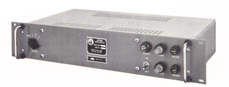
TMC Model AMC-21( ) Solid State Antenna Multicoupler provides low noise optimum distribution of RF signals from 10 KHz to 40 MHz and meets the specifications outlined, independent of the number of plug-in modules selected. Cascading of several multicouplers does not introduce noticeable deterioration.
